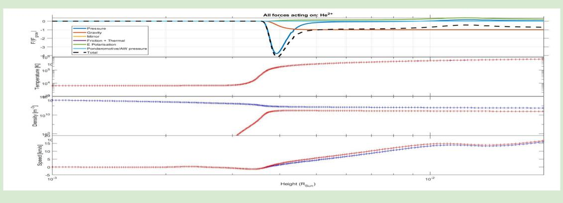
Figure 3 - Forces applying to alpha particles in ISAM model with distance from the Sun. Temperature, density & velocity of protons & alphas is also shown similarly to Figure 2.
