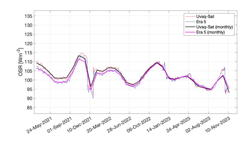
Figure 8. Monthly time series of the TOA outgoing shortwave radiation of ERA5 model with UVSQ-SAT data time acquisition, and UVSQ-SAT (data in orbit) since 2021.
