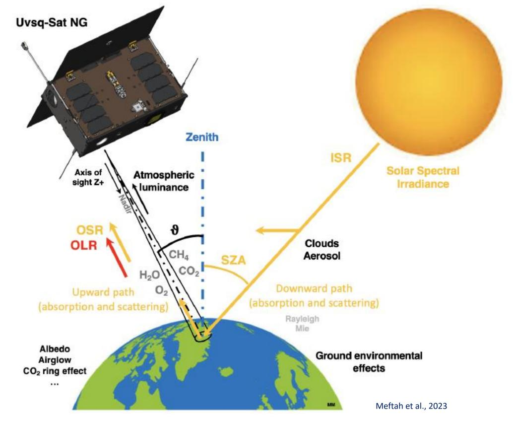
*Figure 2*: Observation approach used by Uvsq-Sat NG to monitor GHG
