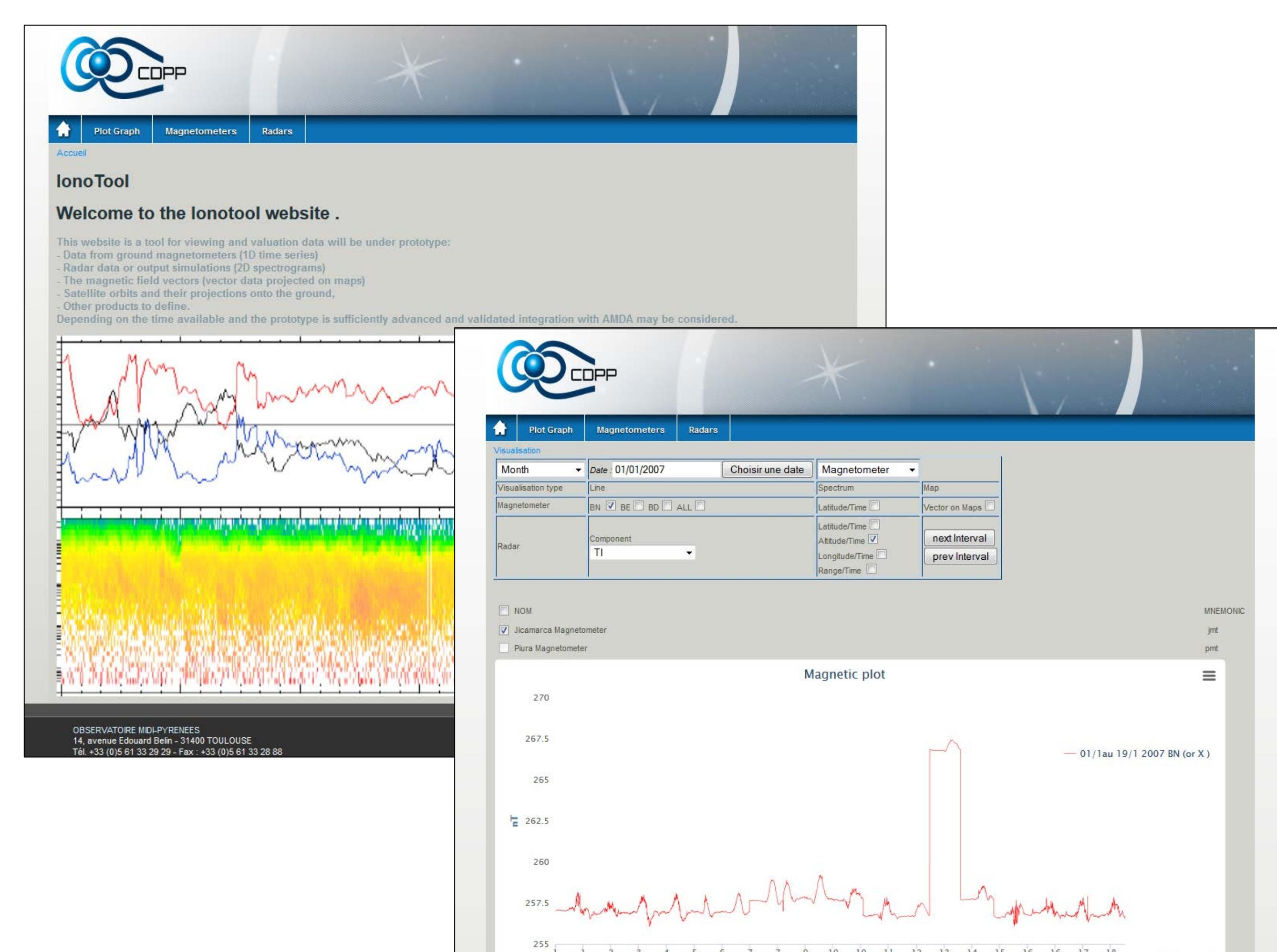
As the prototype is, the user can import magnetometer and radar data from the madrigal data base and plot them as 2D colour plots, time series or altitude profile (when applicable). Alternatively, the user may also export data to AMDA via the SAMP protocol.
